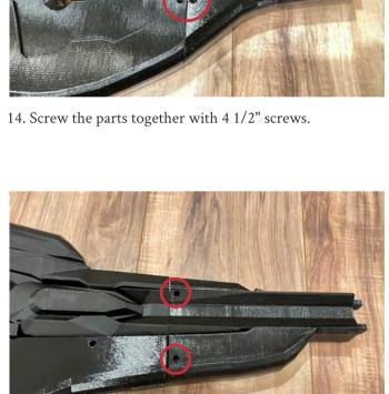
16. Screw the parts together with 2 1/2" screws.
